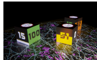
Figure 1: Interactive projection mapping on tangibles on an interactive tabletop.
